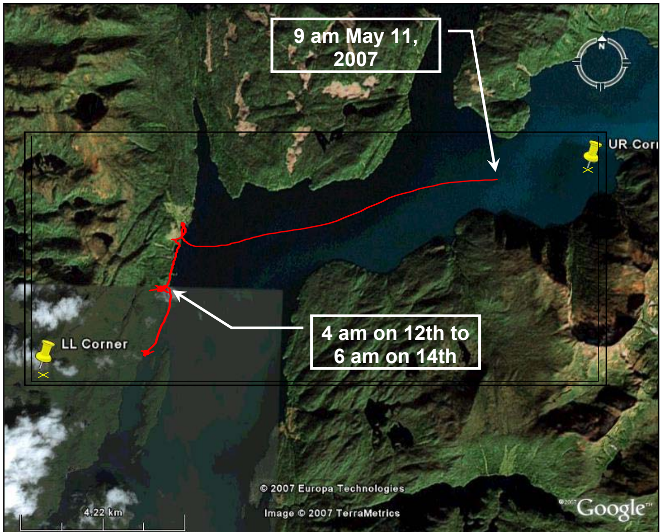
Figure 2. A drifter track superimposed on a Google Earth image of Rivers Inlet. Note how the drifter became hung up on the west shore of the inlet on two occasions. With these anomalies removed, these tracks provide direct observations on the movement of inlet surface waters. These can be compared to predictions of the hydrodynamic model. We hope eventually to be able to use the model to obtain insight on past inlet conditions given local weather and river discharge data, and then to forecast future inlet conditions in light of predicted changes to Central Coast weather in coming decades.
